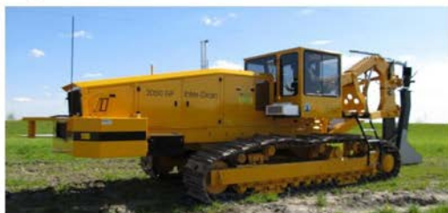
The Inter-Drain plow, three types, double link, single cantilever, or single link, each in three sizes. Cat, Cummins or Volvo power. Offset available.
