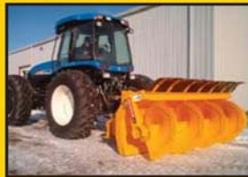
Model PTOAB36-10 for tractors with hydrostatic or creeper type transmission and 100-160 hp
