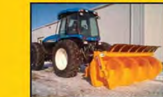
Model PTOAB36-10 for tractors with hydrostatic or creeper type transmission and 100-160 hp
