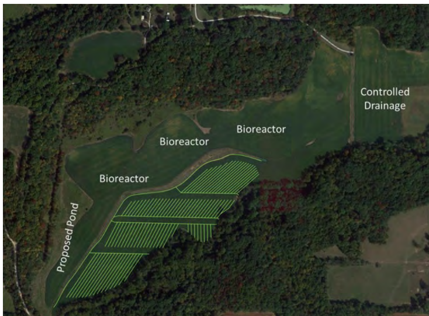
Figure 1. Layout of Drainage Water Recycling Systems at Fulton County Site. Nearby drainage-related management, practices are also identified.
