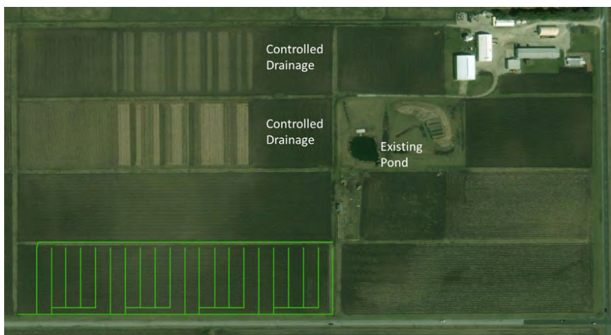
Figure 2. Layout of Drainage Water Recycling Systems at the South Farm Site. Nearby drainage-related management, practices are also identified.
