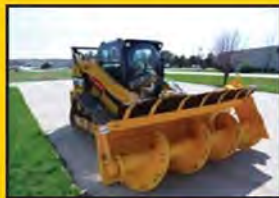
Model R31 for High flow skid and compact track loaders with 3000-5500 psi and 30-50 GPM
