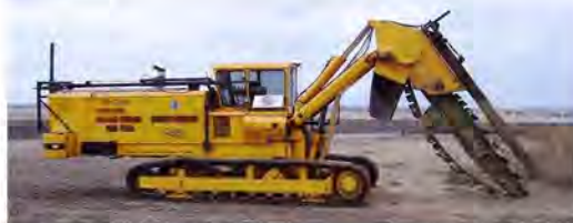
The Inter-Drain chain trencher. Four size choices, mechanical or hydraulic chain drive, vertical and offset available. Cummins, Volvo or Cat power.
