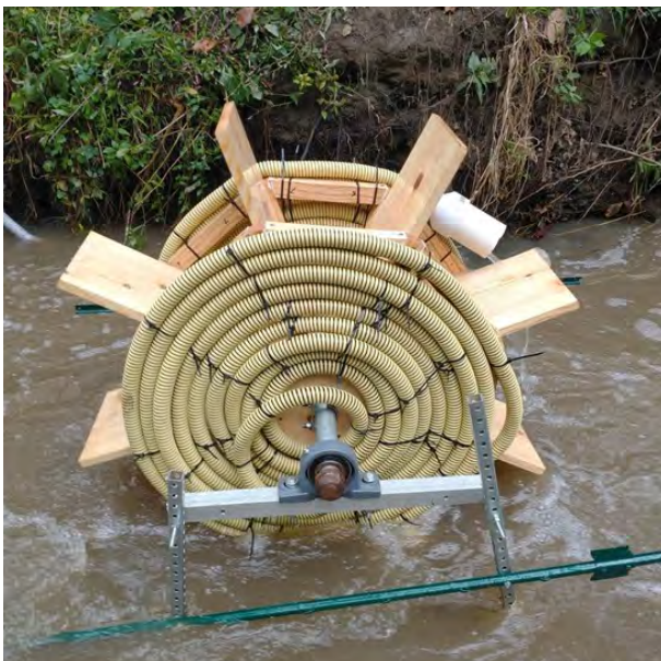
Figure 1. Side view of a 2 feet diameter spiral water wheel in Big Creek, at an experimental site at Fulton County.
