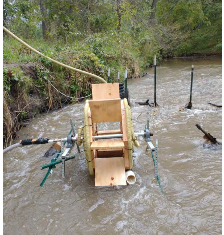
Figure 2. Front view of a 2 feet diameter spiral water wheel in Big Creek, at an experimental site at Fulton County, with the outlet hose from the solar powered pump in the background.
