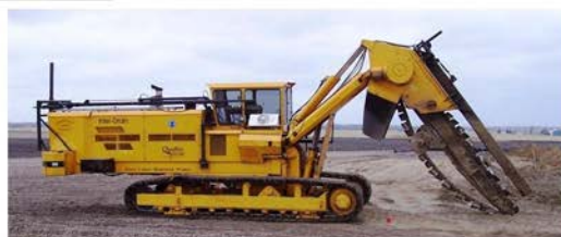
The Inter-Drain chain trencher. Four size choices, mechanical or hydraulic chain drive, vertical and offset available. Cummins, Volvo or Cat power.
