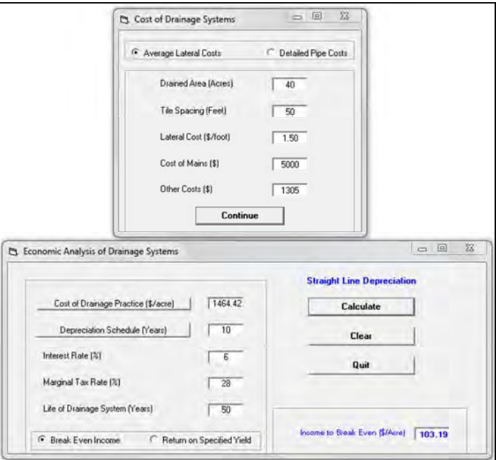
Figure 4. Break even calculation for a scenario with tiles spaced 50 feet apart.
